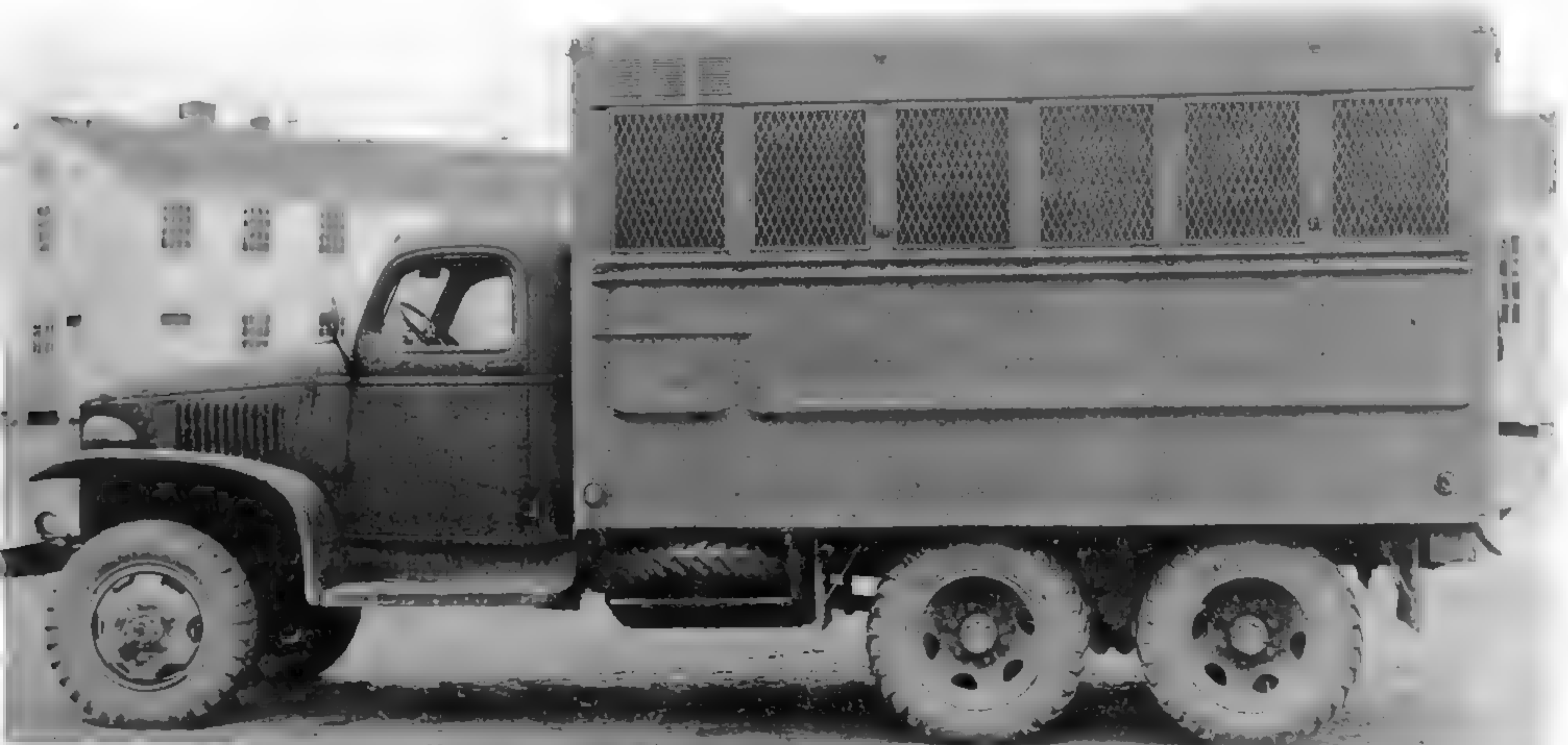
The mobile shop shown here is housed in a model ST-5 bed. This is an early shop truck as evidenced by its closed-cab chassis, chevron pattern tires, and use of the ST-5 bed. Seventeen different types of mobile repair shops were mounted in these type trucks. The ST-5 body was superseded by the ST-6 body. (Photo courtesy of United States Army Engineer School History Office).
